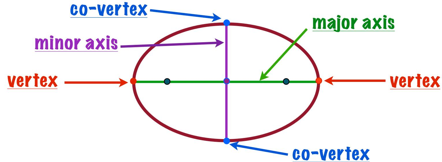
The major axis and minor axis are perpendicular and intersect at the center of the ellipse.
