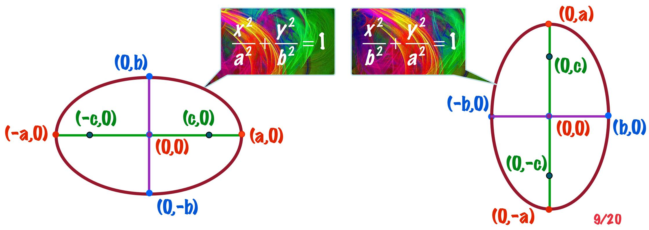
Graph and locate the foci:  $16x^2 + 9y^2 = 144$ Re-write in standard form:  $\frac{x^2}{9} + \frac{y^2}{16} = 1$  Larger Denominator under  $y^2$ Major Axis: Vertical  $a^2 = 16$ ,  $b^2 = 9$  $c^2 = a^2 - b^2 = 16 - 9 = 7$   $c = \pm \sqrt{7}$ Foci:  $(0, \sqrt{7})$  and  $(0, -\sqrt{7})$ Vertices:  $a^2 = 16$ ,  $a = \pm 4$  (0,4) and (0,-4) Co-vertices:  $b^2 = 9$ ,  $b = \pm 3$  (3,0) and (-3,0)
